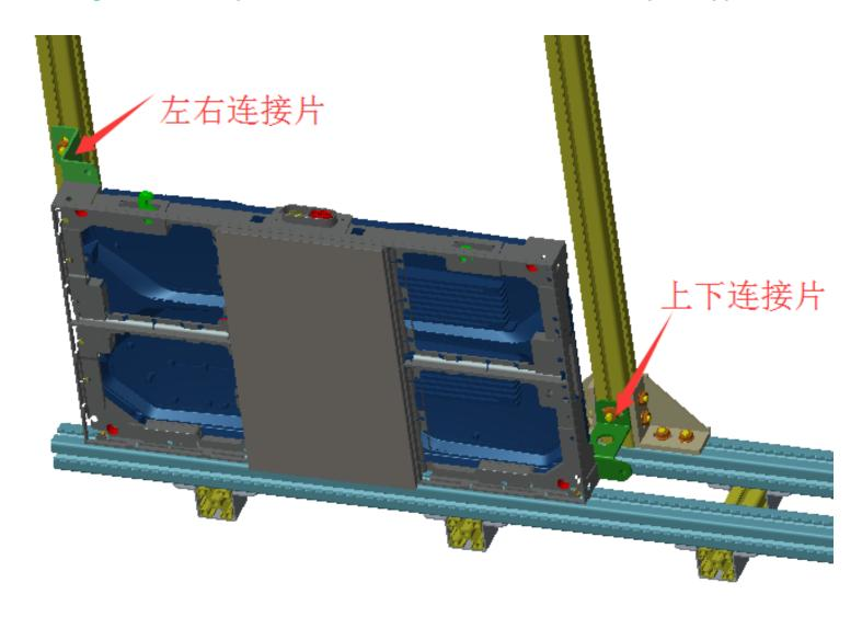
6pcs modules on each cabinet should be took off while installation; What the arrow pointed is to show how to fix the cabinets on the supporting frame; Tighten the M8\*40screw from front side of the cabinet;
