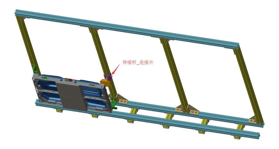
To adjust the connection plates to make sure the screen surface is flat;
