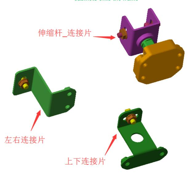
This is the connection plate to fix the cabinets onto the frame; Its flexible and it allows 8mm adjustable horizontally and 10mm adjustable vertically; You can sition;
